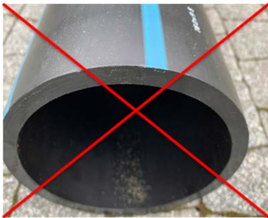
Pipe protected with DBI plug without the membrane (dirt visible)
